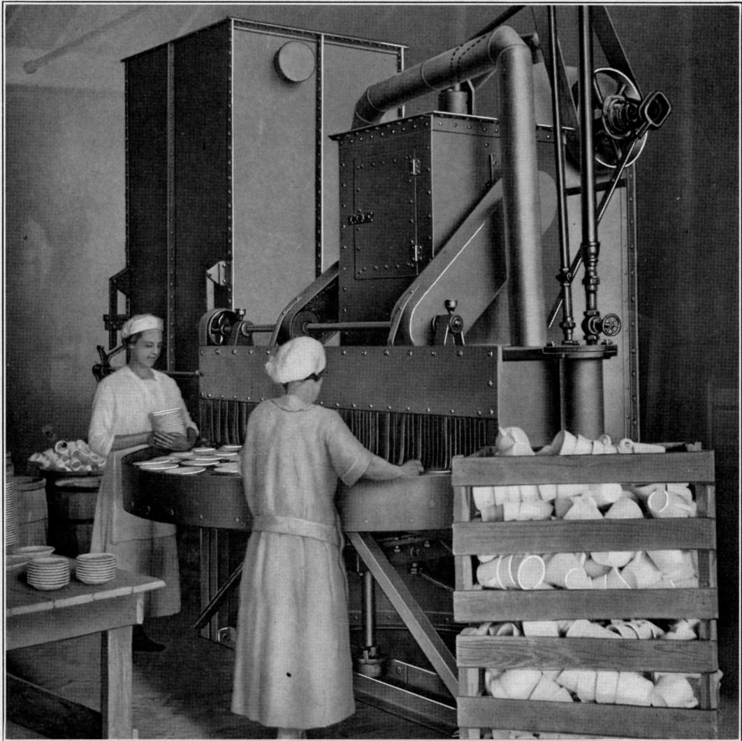
Rotary Table Machine for Cleaning China-ware Connected to an "American" No. 3 Dust Arrester.
